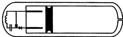
Fig. 1. High frequency controlled drug delivery systems with an energy transmission system, (A) oscillatory circuit (high frequency receiver), (B) drug reservoir, (C) piston and (D) electrolysis chamber with two platinum electrodes.
