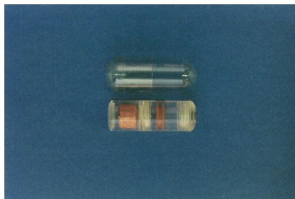
Fig. 6. Photograph of a capsule with a high frequency energy transmission system.
